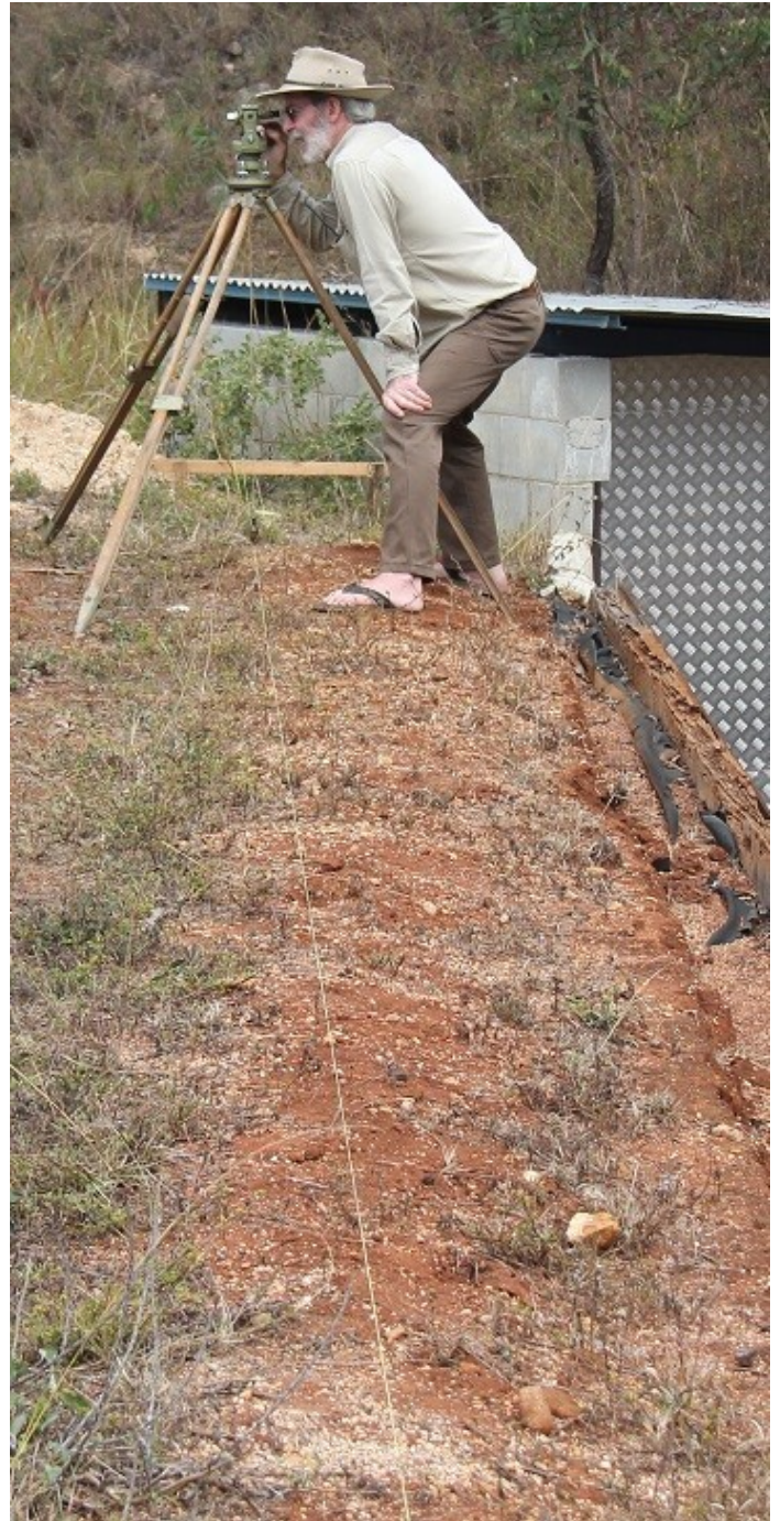
Measuring angles. Line was aligned parallel to target face.
