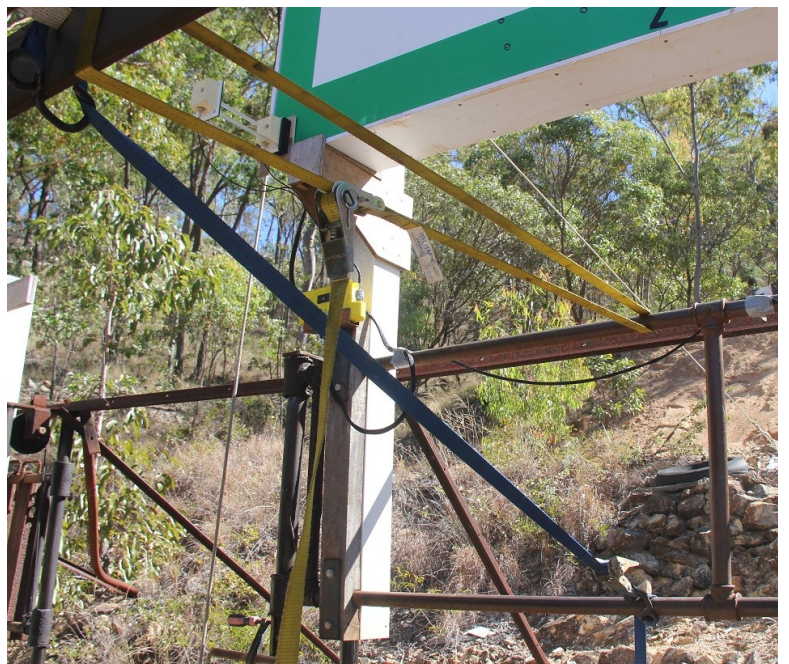
THEY EFFECTIVELY STOPPED ALL TARGET MOVEMENT BACK AND FORTH IN THE LIGHT WINDS EXPERIENCED DURING THE TESTING
