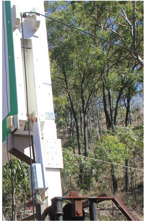
ROPES PULL TARGET FRAME BACK TO VERTICAL POSITION
